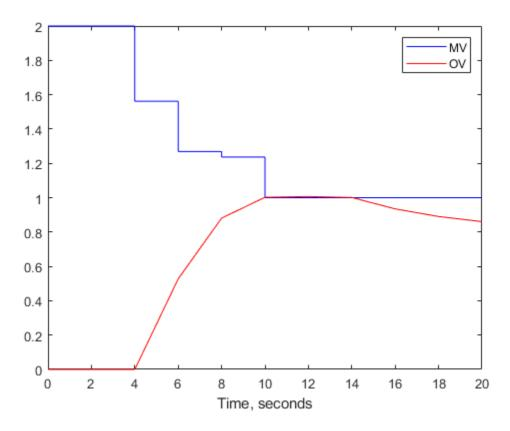
From the plot, you can observe that the original MV upper bound is active until t = 4. After the input delay of 4 seconds, the output variable (OV) moves smoothly to its new target of r = 1. reaching the target at t = 10. The new MV bound imposed at t = 10 becomes active immediately. This forces the OV below its target, after the input delay elapses.
